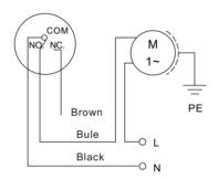
Connect the control's blue line to electric pump, black line is connected to zero-line, brown line can not be connected and should be insulated.
