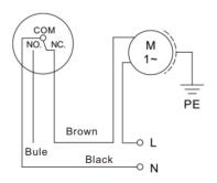
Connect the control's brown line to electric pump, black line is connected to zero-line, blue line can not be connected and should be insulated.
